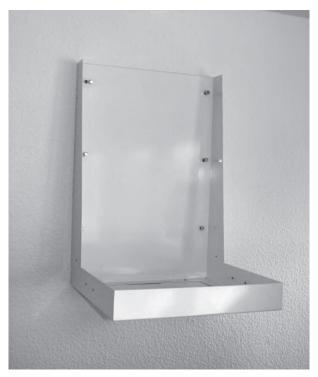
Drill the holes with a 8 mm drill bit and insert the universal wall plugs. Fit the wall screws with the white plastic washers. Position the wall bracket and insert the srews, turning each a few times until it takes grip.
